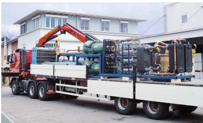
Subject to installation conditions, Viessmann heat pumps are delivered as modules.
