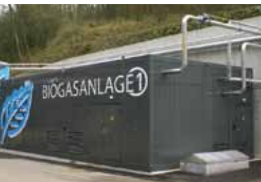
The raw gas for the upgrading plant in Bern (Switzerland) is yielded from sewage gas and waste.
